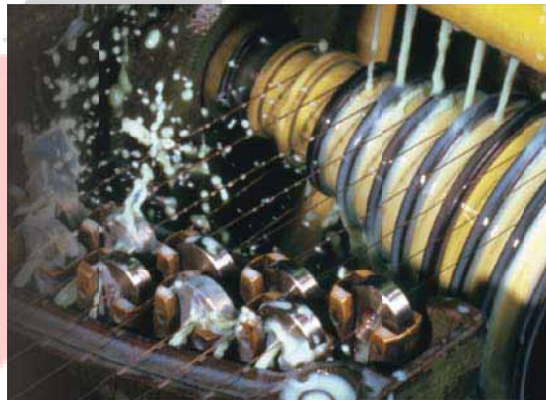
Wire drawing extrusion tips & dies For extruding insulating materials over wire, cable and fiber-optic cable
